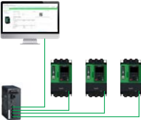
Firmware upload of several ATS490 soft starters at the same time through Modbus TCP/EtherNet/IP or Modbus serial using Ecostruxure Automation Device Maintenance
